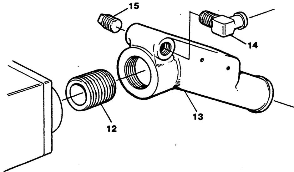
WESTERBEKE 40A - FRESH WATER PUMP AND WATER INJECTED EXHAUST ELBOW
