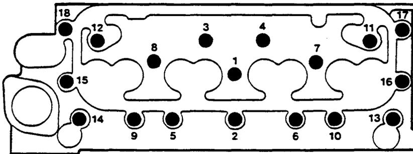
3. Torque the rocker shaft bracket securing nuts evenly between 12 to 15 lb-ft or 1.7 to 2 kg-m.
