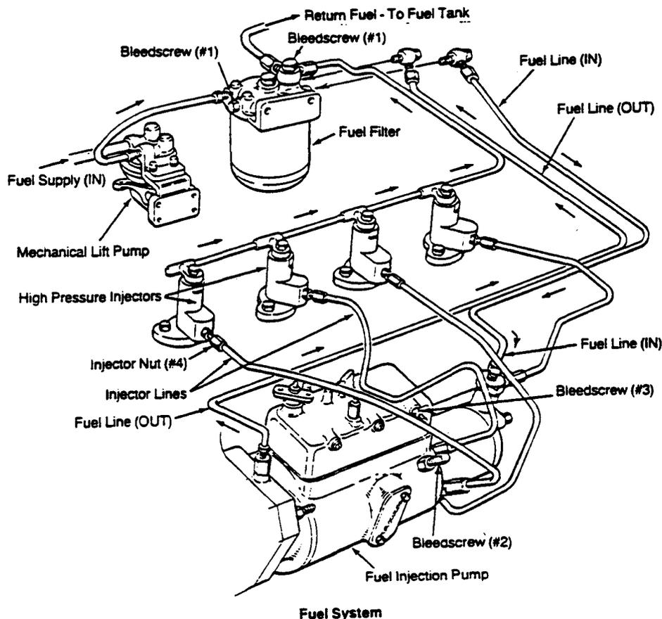
4. Using the 5/16" box wrench or the 1/4" drive 5/16" socket wrench, open the #3 bleed screw and bleed this portion of the fuel injection pump in the same manner as described in step #3. Proceed to step #5
