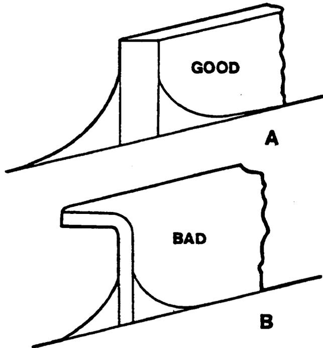
**Note:** Avoid excessive height, use solid stringer construction (A).
