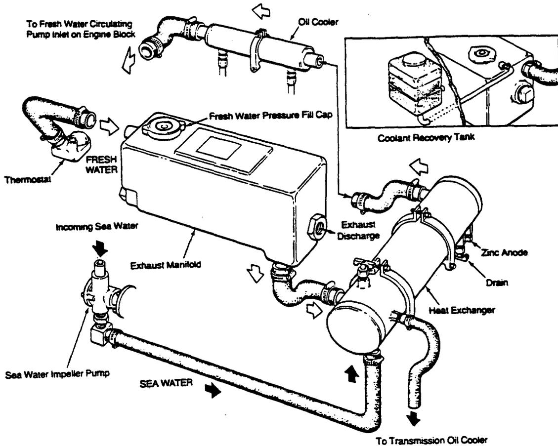
Illustrated above is the cooling system for the W 40NA engine
