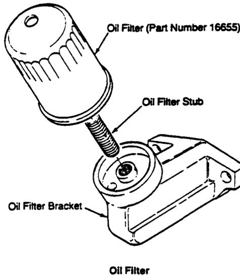
When installing the new oil filter element, wipe the filter gasket's sealing surface on the engine block free of oil and apply a thin coat of clean engine oil to the rubber gasket on the oil filter. Screw the filter onto the threaded oil filter stub, and then tighten the filter firmly by hand. See the "TORQUE SPECIFICATIONS" section of this manual for the proper oil filter tightening specification, page 61.
