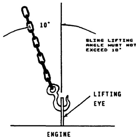
The general rule in moving engines is to see that all of the equipment used is amply strong and firmly fixed in place. Move the engine a little at a time and see that it is firmly supported. Eliminate the possibility of accidents by avoiding haste. Do not lift the engine by its propeller coupling, or pry against this coupling with a crowbar, because excessive pressure of this type may distort the coupling.
